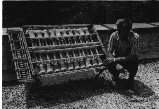
Figure 9.- Stressed exposure rack.
